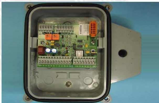
single loop detector ESD in a line side box
